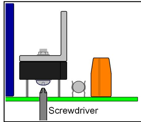
Wires may be soldered directly to the PCB, or you can use screw terminals if you like. Direct soldering saves a few dollars and potentially increases reliability, as screw terminations may be prone to loosening in a high vibration/movement environment such as may be found on the road.
